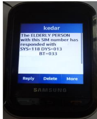
Fig.4 Photograph of a Mobile phone with SMS sent by the Wearable unit
