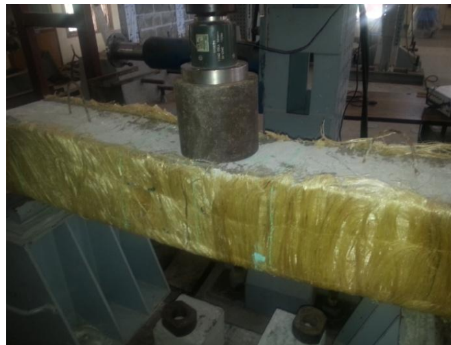
Fig. 5 Typical view of Specimen Retrofitted with SISAL fiber sheet
