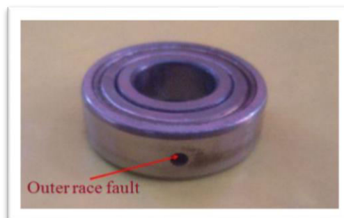
Figure 3: Outer race fault
