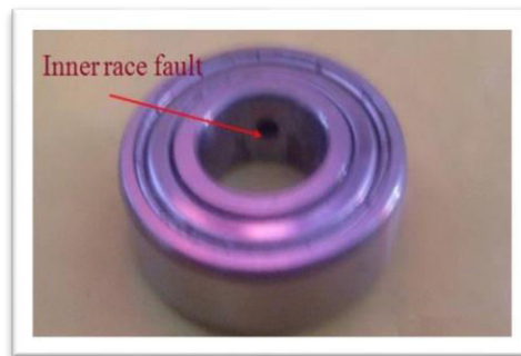
Figure 2: Inner race fault
