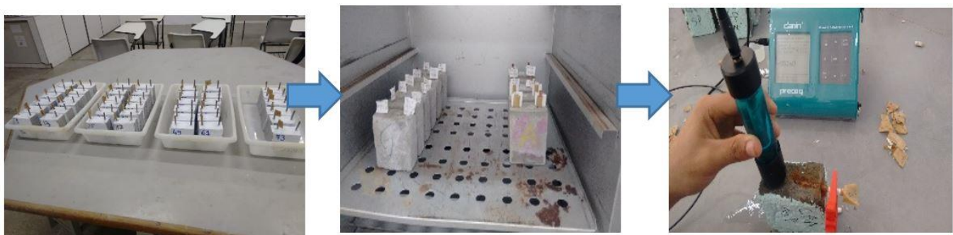
Figure 2. Induced corrosion test: NaCl solution; oven 50°C; Measurements of potentials.
