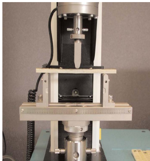
Fig -1 Three point bend test on composite specimen
