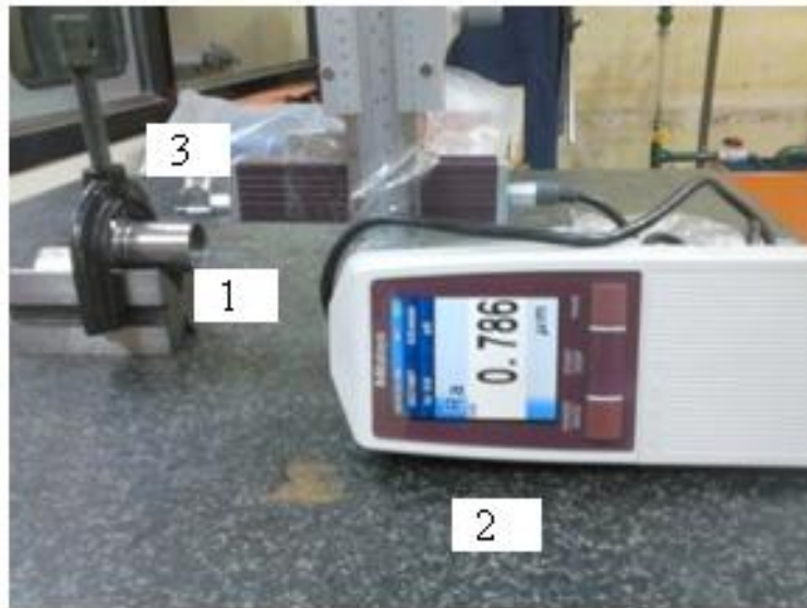
1. Component 2. Mitutoyo Surface Roughness Tester SJ-201 3. Stylus Figure 6: Photograph of Mitutoyo Surface Roughness Tester.
