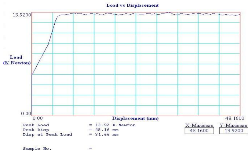
Fig. 5.3 Bending result generated by UTM (composite material with hexagon)
