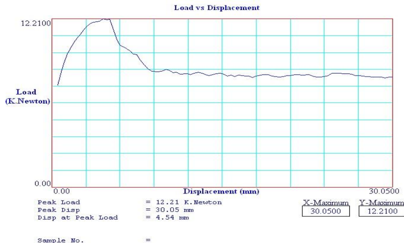
Fig. 4.5 Tensile result generated by UTM (composite material with hexagon)
