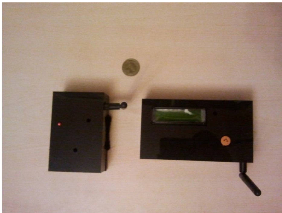
Fig.4 The final result of soldier unit and operation unit in the designed covers
