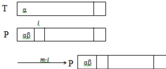
Figure 2(a): a of text T is present in pattern P , so shift by m-i
